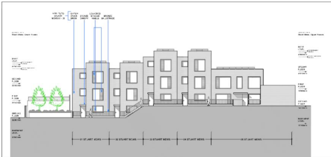
Figure15: - Mews units inner facing elevation
